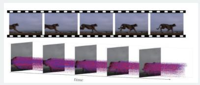
Event camera. The normal camera frame above causes motion blur and insufficient frame rate. In contrast, the red and blue event data below represent asynchronous high temporal resolution luminance changes per pixel. https://w.wiki/5JKV
